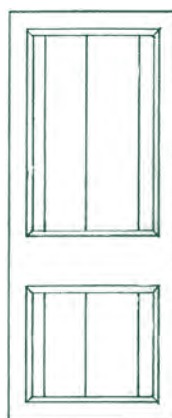
A framed and boarded door with butt-jointed boards nailed to back of frame.
